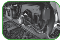
Bogies / under carriage
